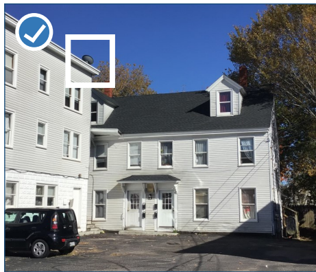
Figure 131: Appropriate location for satellites and antennas on the rear elevation of a residence.
