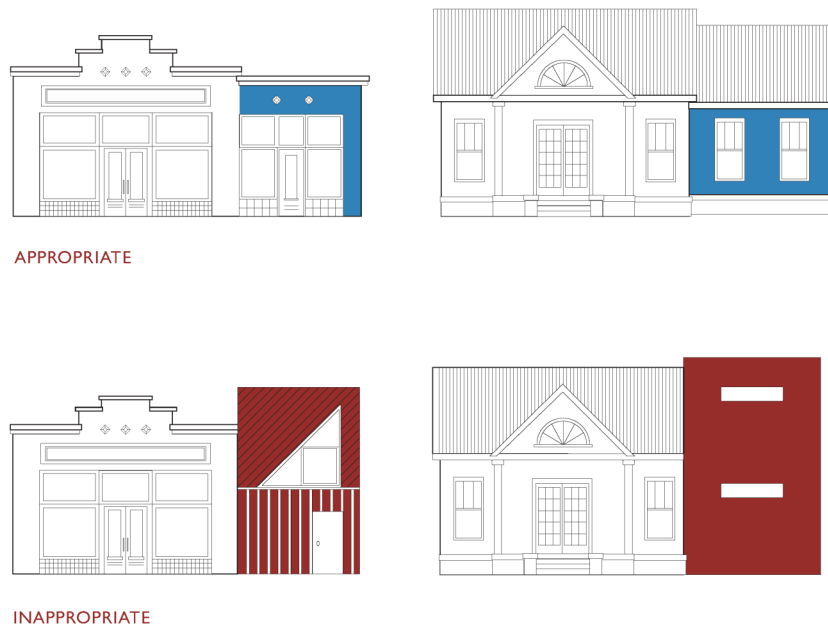
Figure 140: Diagram of the appropriate and inappropriate scale and fenestration of side additions.
