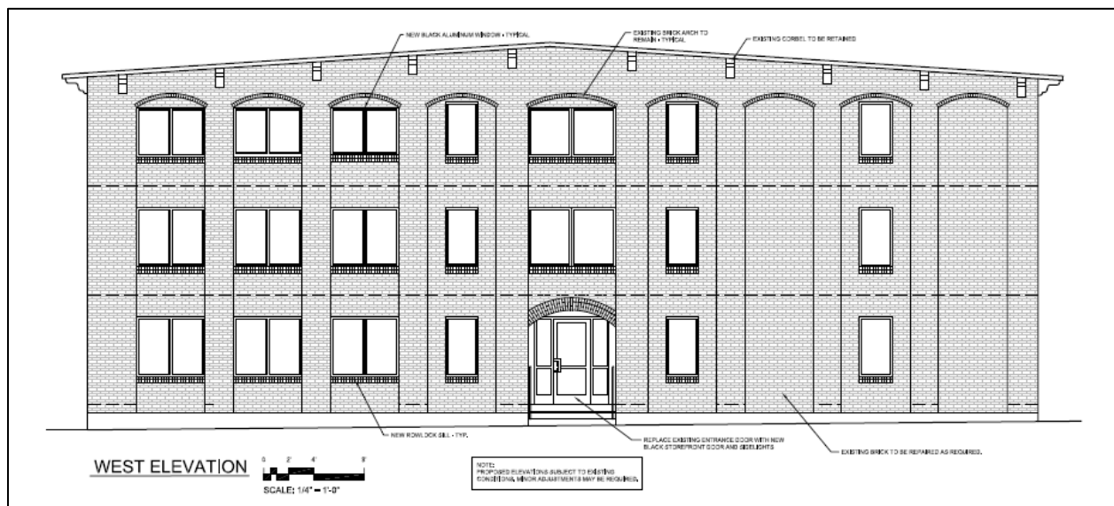
West Elevation. Note new storefront entry at center bay and new windows installed in bays currently solid (no portals) at left side of building.
