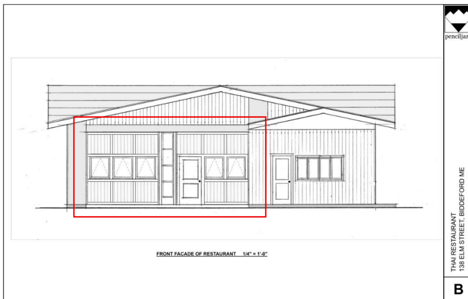
B. T-111 with lines to imitate the old garage doors
