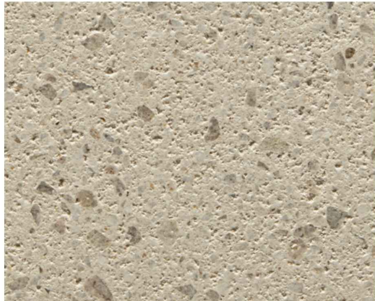
GROUND FACE CMU BASE
