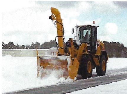
Front End Loader with Snow Blower Chatham Municipal Airport
