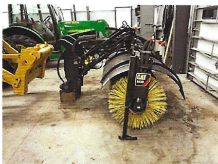
Broom Attachment for Loader Chatham Municipal Airport
