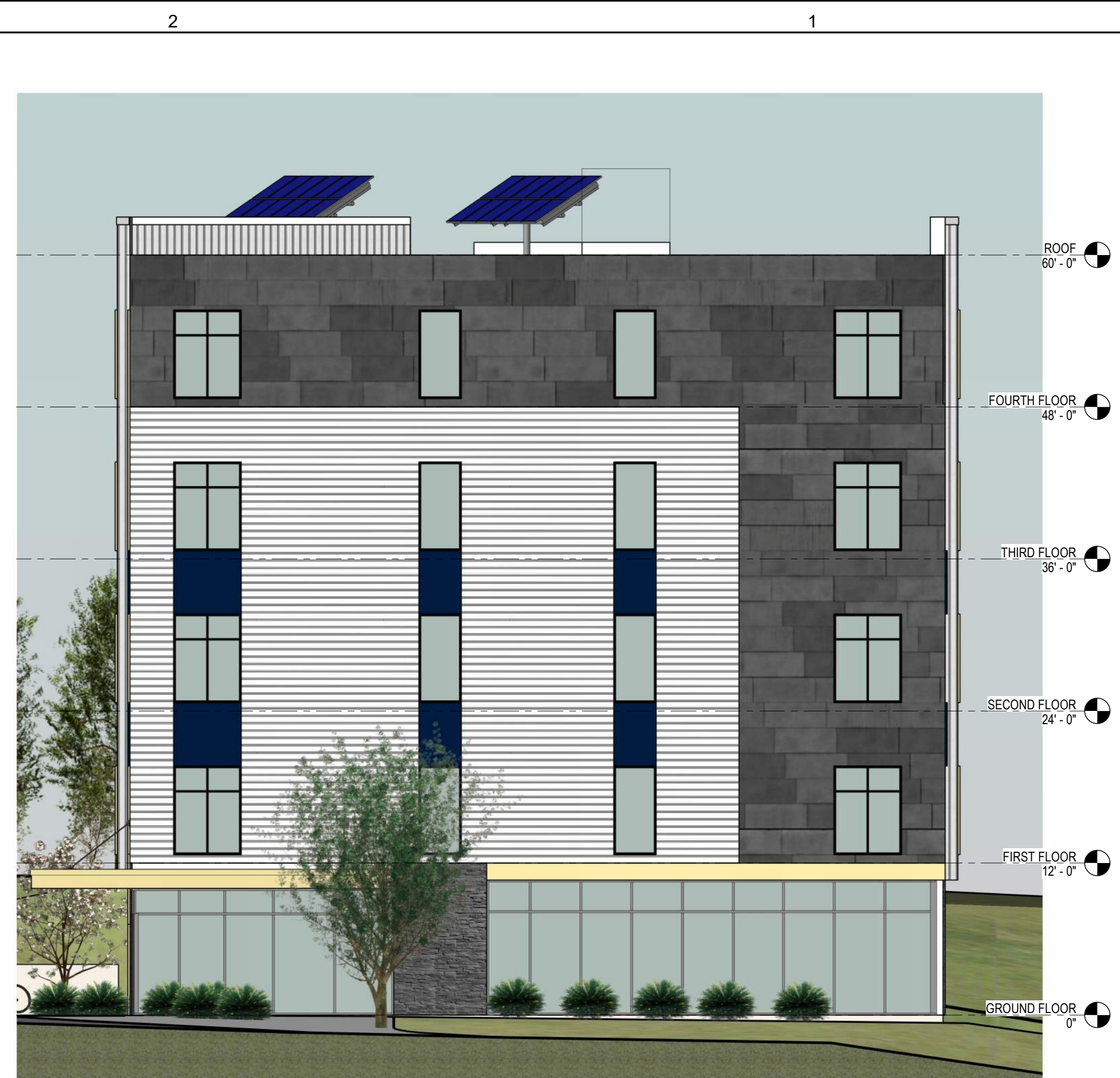
2 EXTERIOR ELEVATION - EAST 1/8" = 1'-0"
