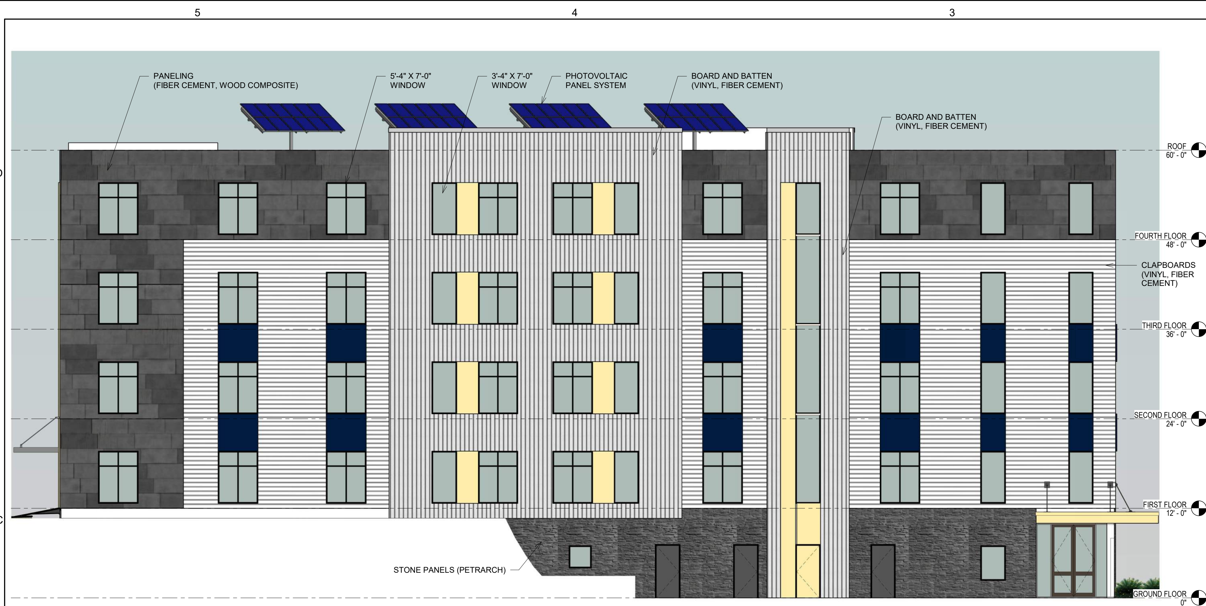
1 EXTERIOR ELEVATION - SOUTH 1/8" = 1'-0"
