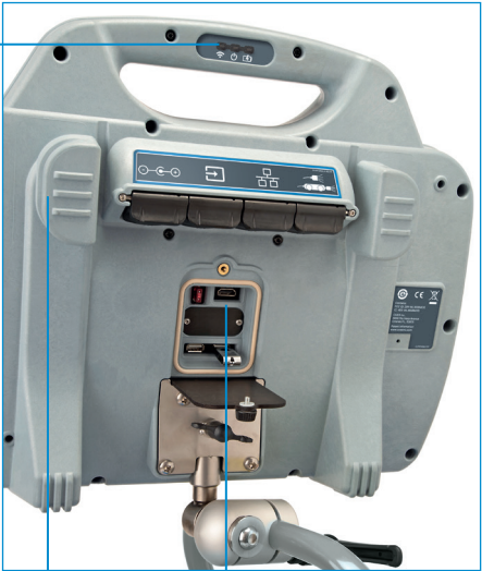
Convenient cable-tidy hooks Connectivity: USB, HDMI, WiFi, ethernet, audio and analog video in
