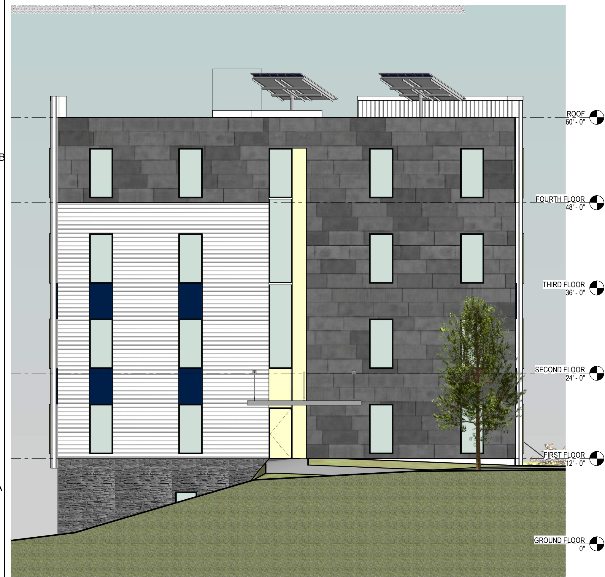
3 EXTERIOR ELEVATION - WEST 1/8" = 1'-0"
