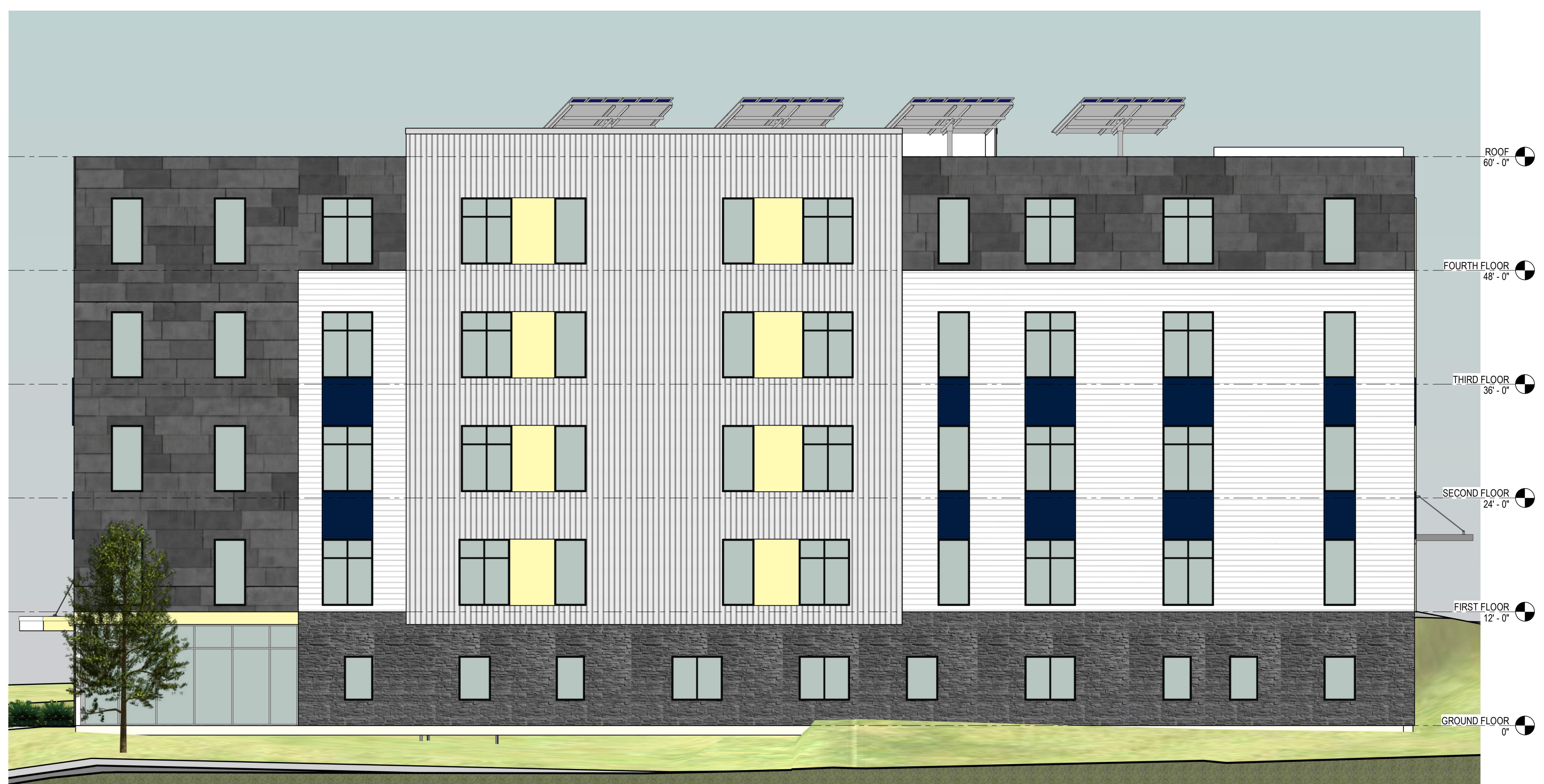
4 EXTERIOR ELEVATION - NORTH 1/8" = 1'-0"
