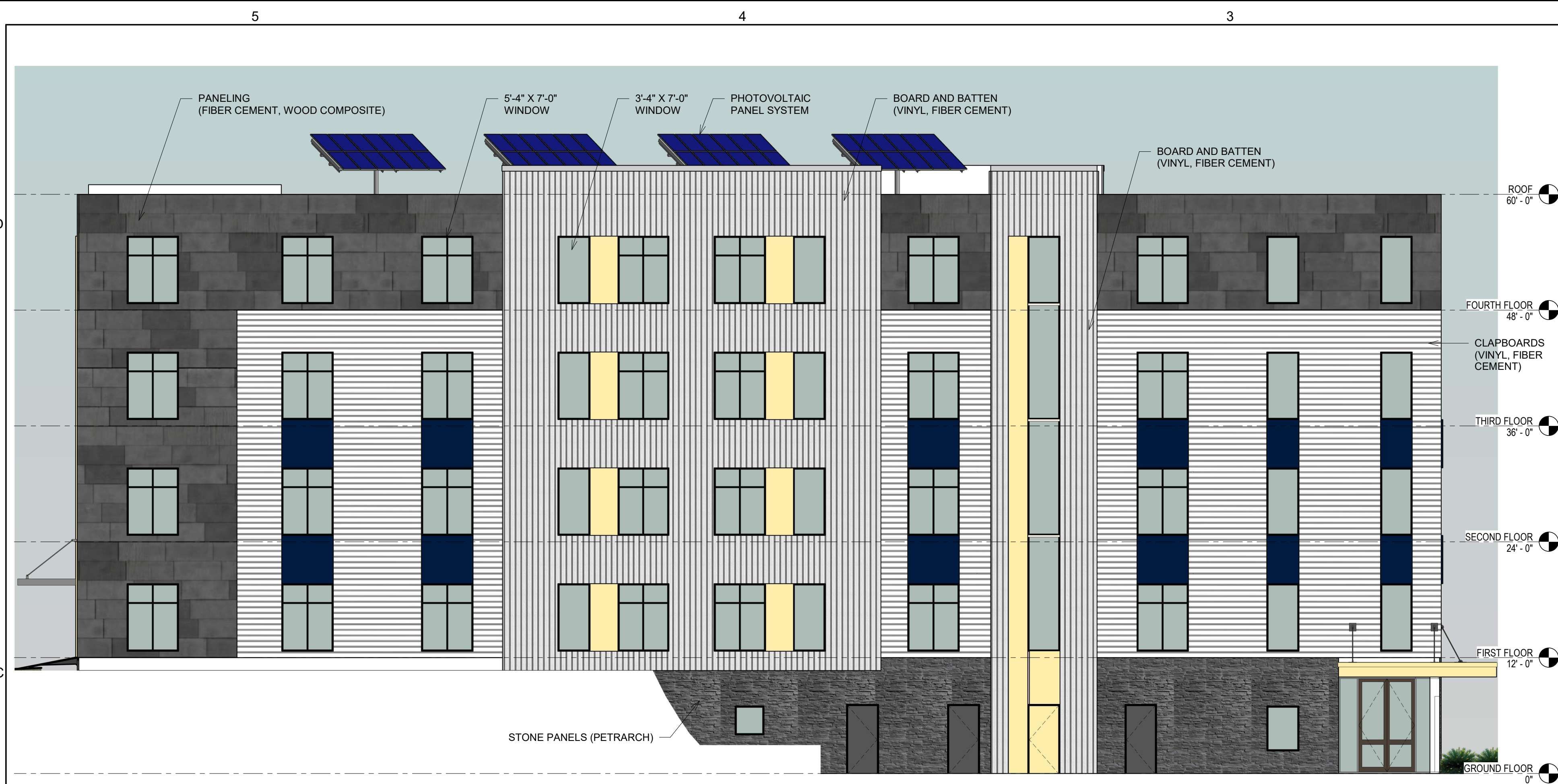
1 EXTERIOR ELEVATION - SOUTH 1/8" = 1'-0"
