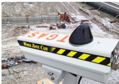
Site Camera, "TGAS1" recorded this image of the steel frame of our EMS Facility at 3PM on 02.28.15. Hourly images are sent to our server throughout the duration of the project.
