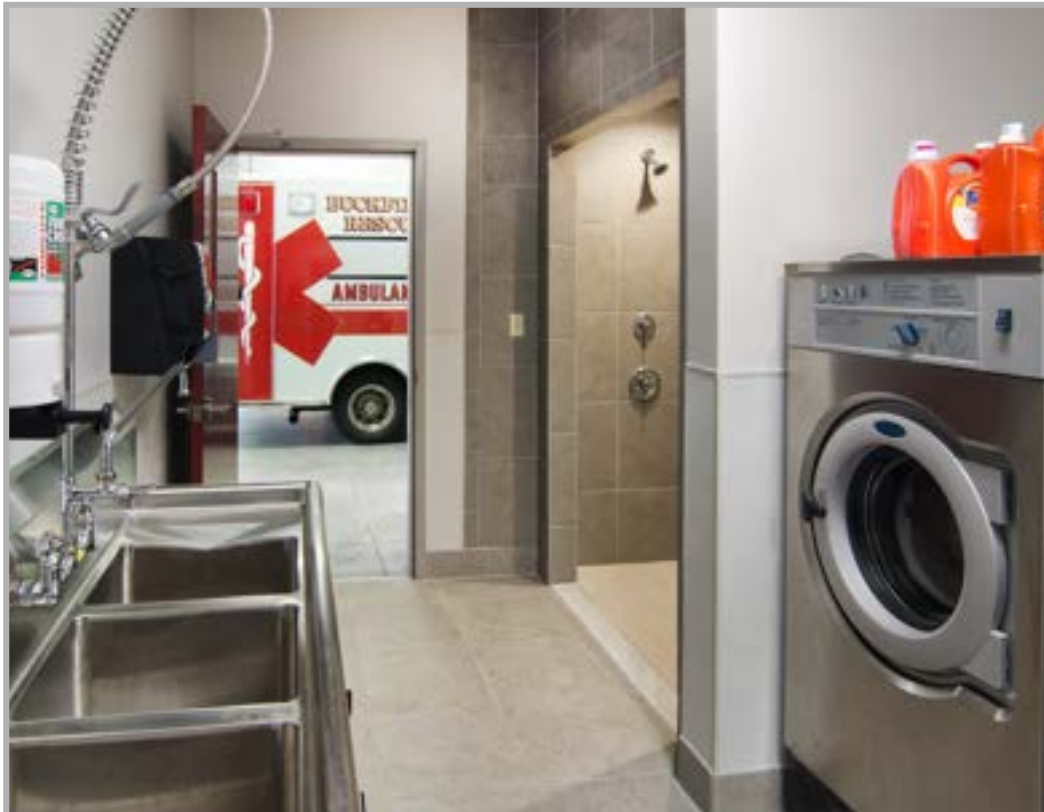
Decontamination Room: A walk-in decontamination shower allows for stretcher boards and other large items to be washed.
