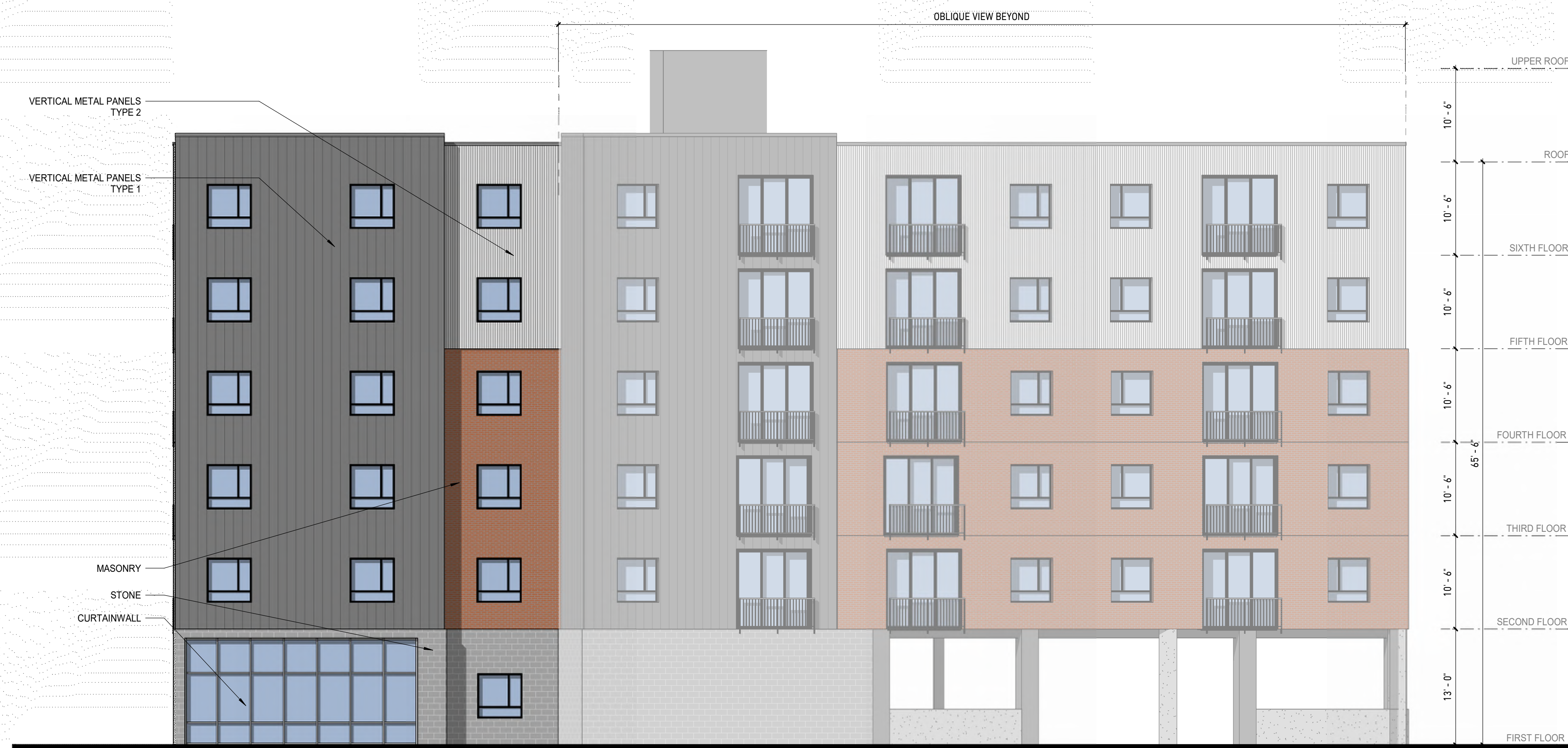
OVERALL NORTHEAST ELEVATION \frac{1}{8}" = 1'-0" B3
