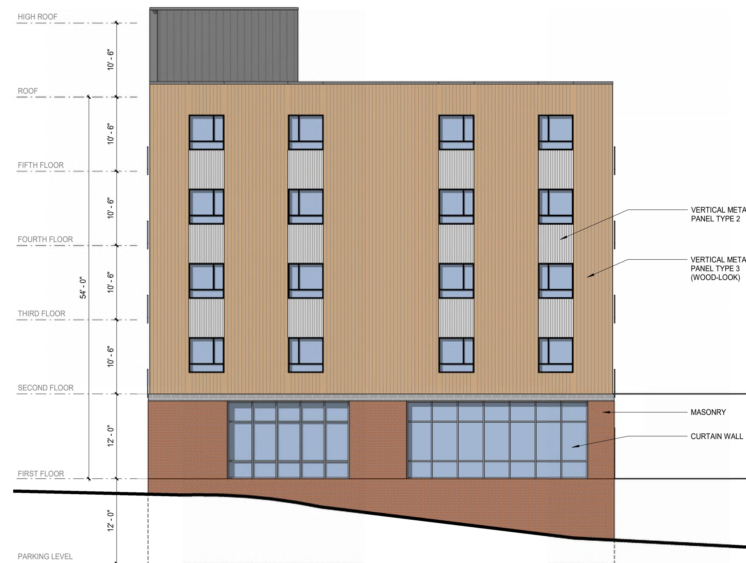
C OVERALL NORTHEAST ELEVATION A2 1/8" = 1'-0"
