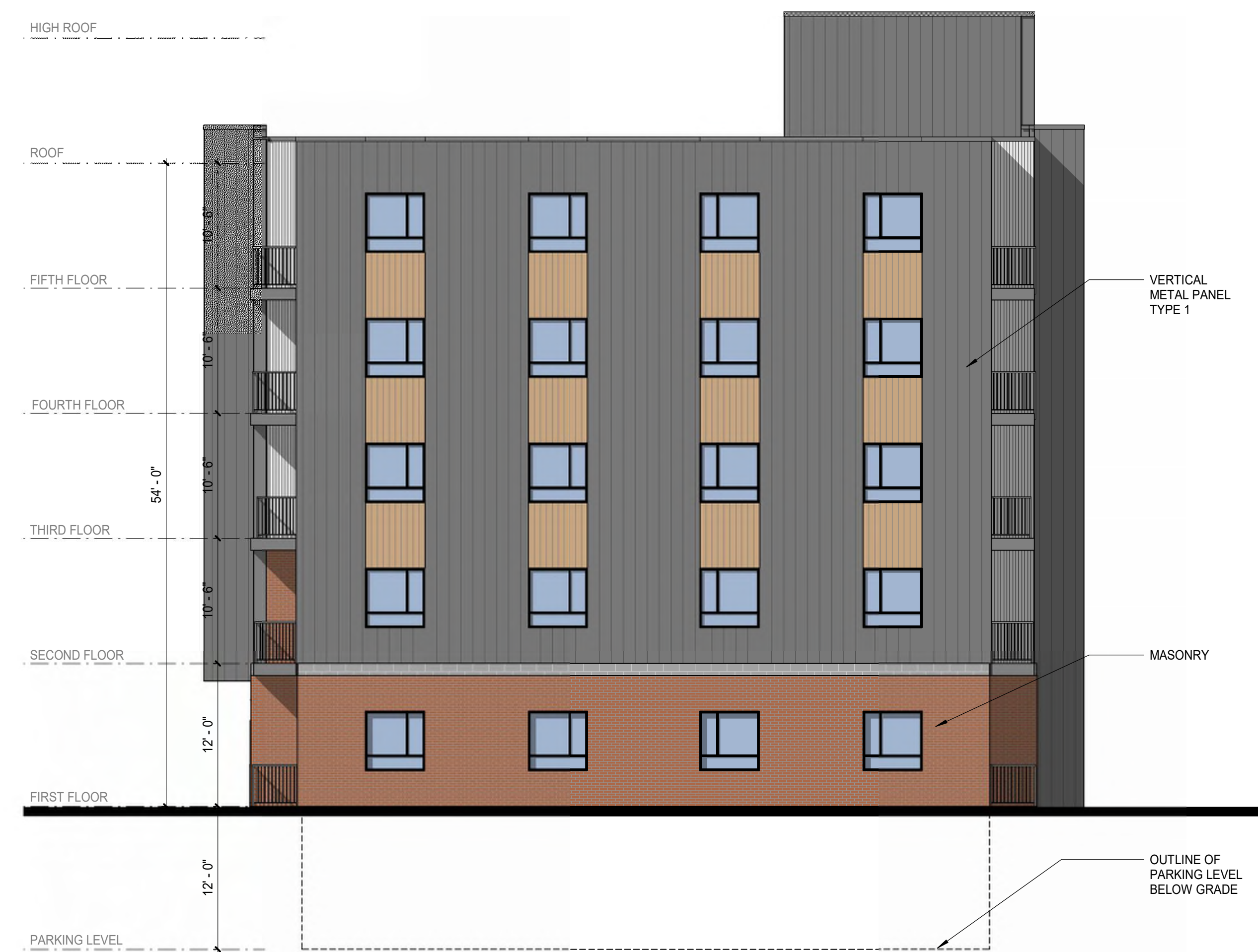
C OVERALL SOUTHWEST ELEVATION A2 1/8" = 1'-0"
