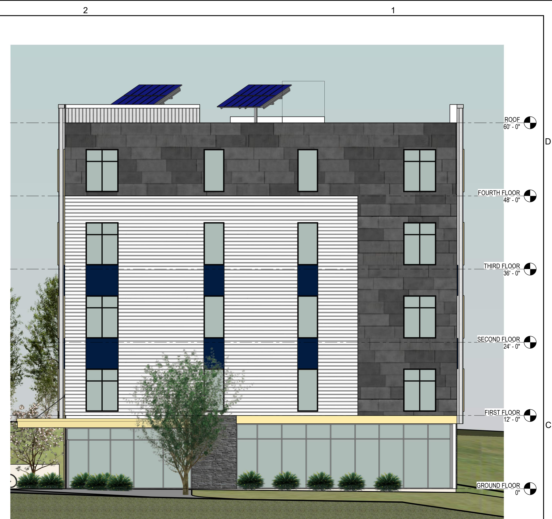
2 EXTERIOR ELEVATION - EAST 1/8" = 1'-0"
