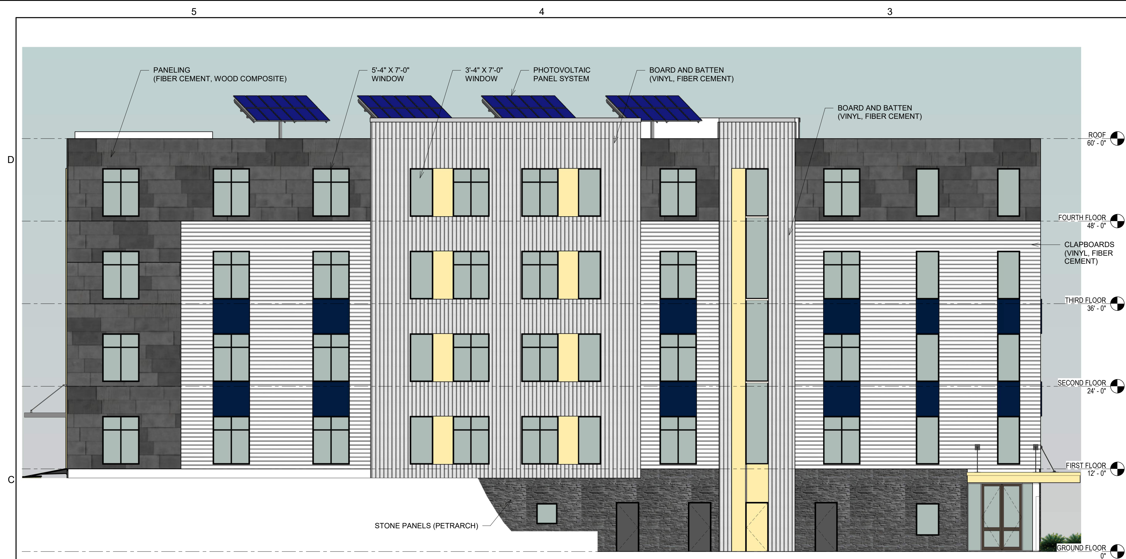
1 EXTERIOR ELEVATION - SOUTH 1/8" = 1'-0"
