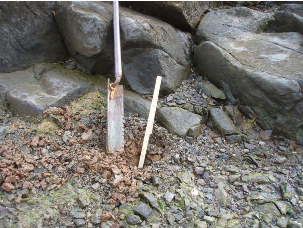
Photograph Nine. Photograph of the very rocky and shaly like soil materials intermixed with the ledges. This picture is within the proposed seasonal pier alignment. Photograph date: 03/13/2023.
