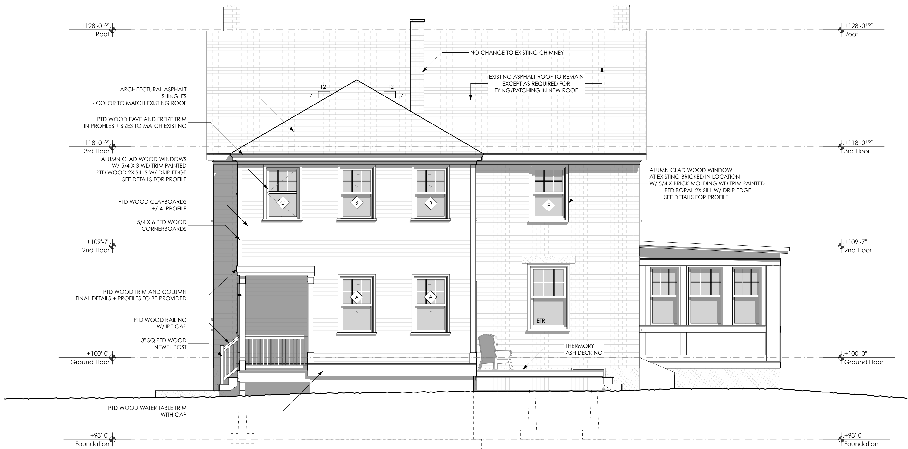
1 PROPOSED- WEST ELEVATION SCALE: 1/4" = 1'-0"
