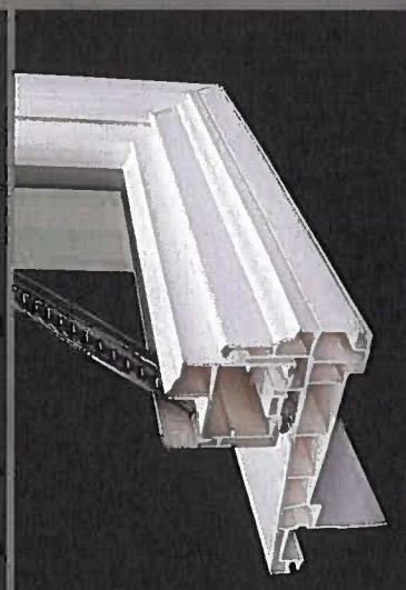
Our Patented Sash Glazed Double Hang Picture Window provides the exact same sight line maintained within the same glass planes as our operable Double Hang units. This provides an aesthetic improvement over current window designs. Our Historic 1854 Ovoid Sticking (on 3" glazed sash), Putty Bead contours as well as the radius edge on the Sill Dam maintain the historic accuracy. With Performance Grade 50 ratings the Sanford Hills is as rugged as it is beautiful.
